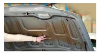
**Step 2: Locating the mounting clip sockets** Identify all the places where you will attach the clips. The mounting holes in the bonnet align with the gaps in the insulation, making it easier to fit.
