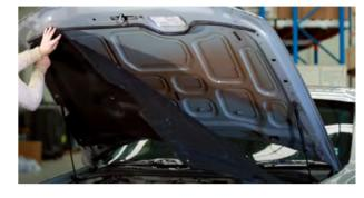
**Step 3: Placing the insulation** Place the hood insulation in the place where you want to fit it. Make sure it matches and covers the area to be insulated.
