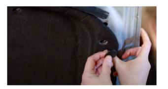
**Step 4: Attaching the clips** Position the insulation so that the gaps match the sockets in the hood.
